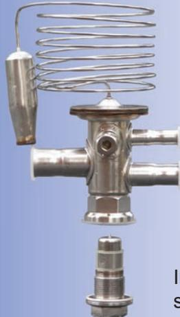
SS Thermostatic expansion valve that modulates refrigerant flow to match system requirements in fluctuating ambient temperatures and compressed air loads. Capillary tube systems used by other manufacturers will increase or decrease refrigerant flow on ambient conditions with no regard to system load. High ambient temperatures or slightly clogged condensers will increase refrigerant flow without a load to balance the system. Operation under these conditions can cause premature compressor failure.
