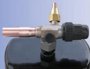
ERF series dryers are equipped with full service refrigeration valves on both the suction and discharge systems. These valves simplify field maintenance or service as well as reducing refrigerant loss.
